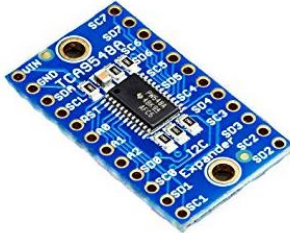
TCA9548 A Low-Voltage 8-Channel I2C Switch
