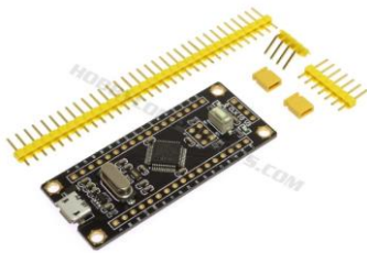
STM32F103C8 Mainstream Performance line, ARM Cortex-M3 MCU with 64 Kbytes Flash, 72 MHz CPU, motor control, USB and CAN
