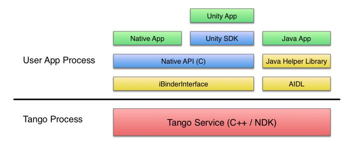
TangoService is an Android service running on a standalone process. It uses standard Android Interprocess Communication to support apps written in Java, Unity, and C. TangoService performs all of the main Tango technologies, such as motion tracking, area learning, and depth perception. Applications can connect to TangoService through APIs. We chose to work with Unity SDK which is great for making games and other programs requiring 3D visualization.
