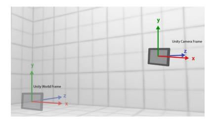
Converting Tango Pose data into the Unity Coordinate System
