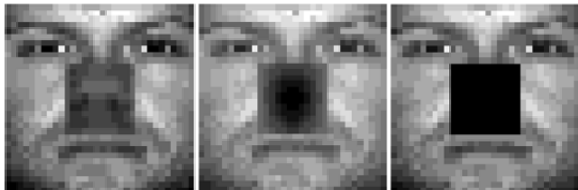
Figure 3 : Initialization strategies for the algorithm. The right-most is the corrupted image to inpaint. The left-most is initialized with the average image referring to all the examples
