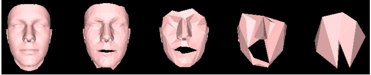
Figure 1. QSlim mesh down sampling
