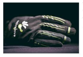
to precisely detect a wide variety of hand and finger movements. These gestures are translated into control commands which are sent directly to connected devices.
