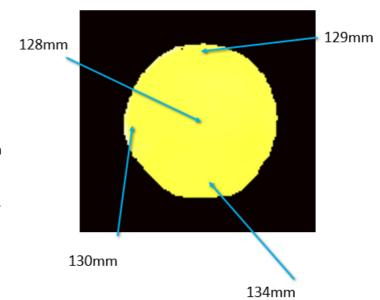
We needed to find somehow a way to tell whether a can is standing or laying (because of the different ways to handle it). Thus we tried a couple of methods to differentiate between laying and standing can:
