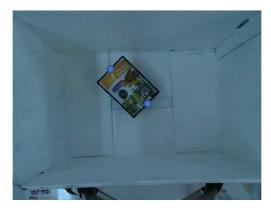
If the can is laying fully down, theses points describe the curve itself, and they are the points that will be returned. But, for tilted cans, we need to first find the most upper point on the curve between the two midpoints:
