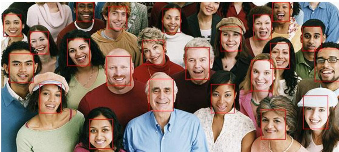
From our experiment it ranges of detection from a regular laptop computer is around ~9 meters. When detection of faces that are further starts to become unstable.
