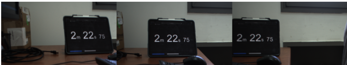
Figure 4: Visualization of the HW triggering mechanism - All three cameras trigger at the same time.
